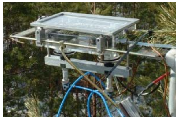
7. Measuring carbon dioxide uptake rates of trees (here by a branch cuvette in Hyytiälä / Finland) is much more uncertain than measuring the relatively stable CO 2 mixing ratios in the air. Source: University of Helsinki
