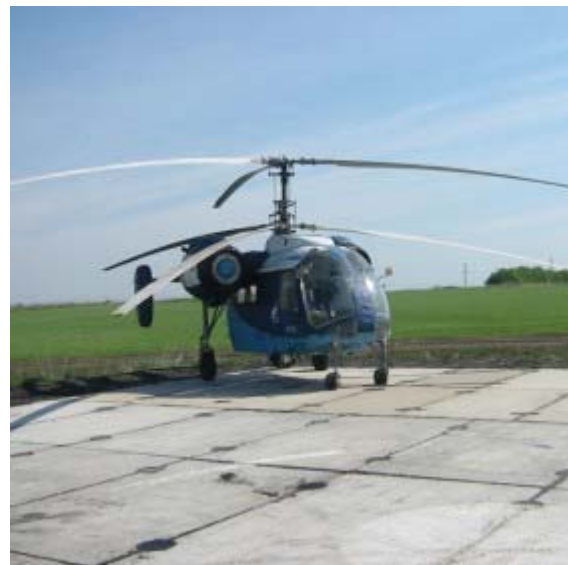
12. A small helicopter is used to check the air along the pipeline with a laser detector. © LA
