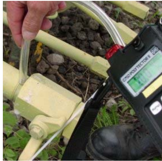
10. Check with a methane detector
