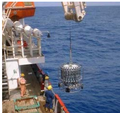
6. a + b) CTD sampling: In order to learn more about the life in the ocean scientists takes samples. The sampling vessel measures Conductivity, Temperature and Depth (CTD) and is equipped with 12 or more sampling bottles which can collect water samples, including the organisms from different depths in the sea. Photo top: NASA, bottom: Tom Bell.
