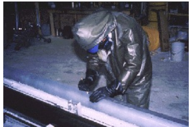
Markieren von Eisbohrkernen Foto: Climate Change Research Center - University of New Hampshire
